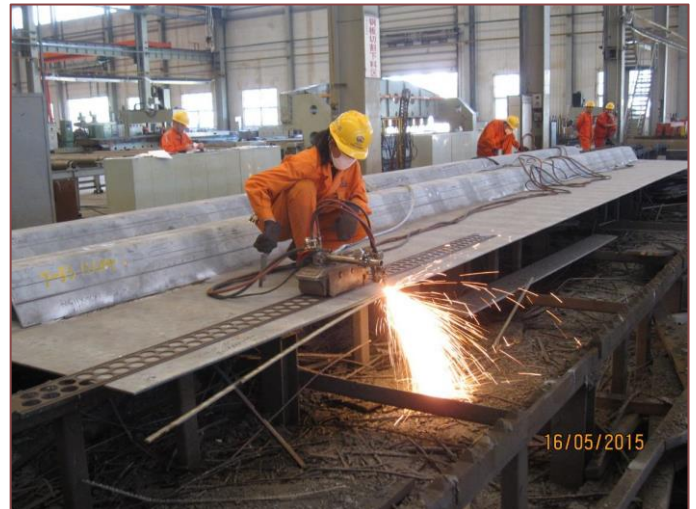
Figures 23 +24: Steel deck segments prefabrication in a workshop
