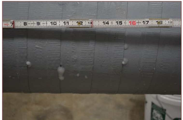
Figure 19. Soapy water inspection of cable wrap on shop test rig (note the bubbles indicating air leaks in the overlap areas)
