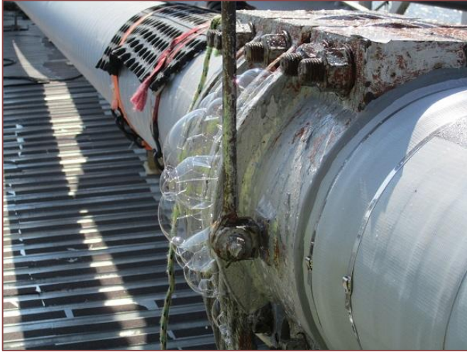
Figure 16: Air trials with soapy water test on in-situ cable band (note bubbles detecting leaks around cable band bolts and suspender ropes)
