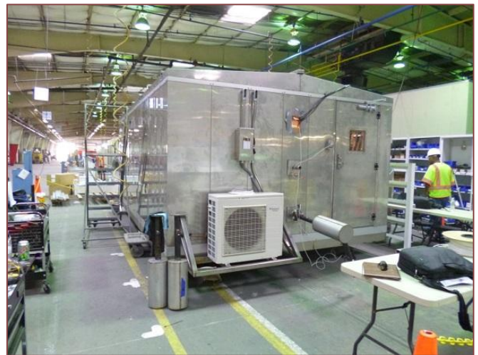
Figure 21: Eastbound Bridge plant room preassembly and shop commissioning
