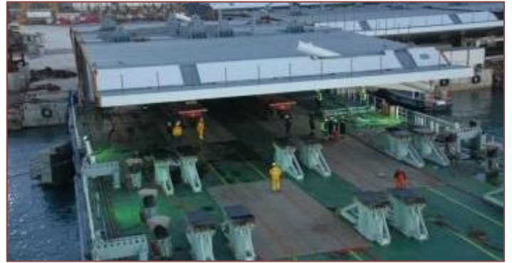
Figure 8: Customised supports with special anti-slip mats on top & buffering system to compensate vertical movements during lifting operations
