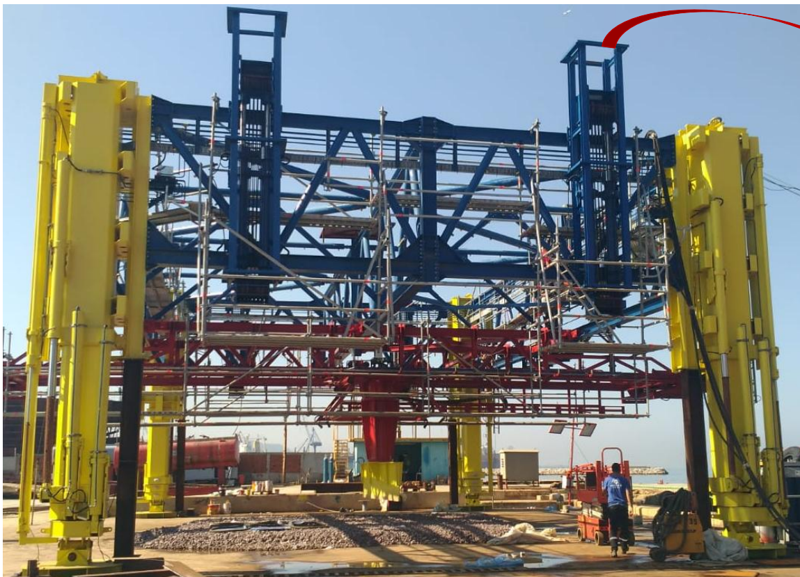
Figure 5: Hydraulic cylinders on the main body
