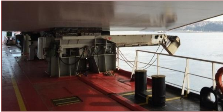
Figure 7: Remote controlled foldable lashing arms to ease unlashng and increase operational safety at sea
