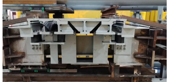
Figure 5: LR3-FE fuse break-away test – before break
