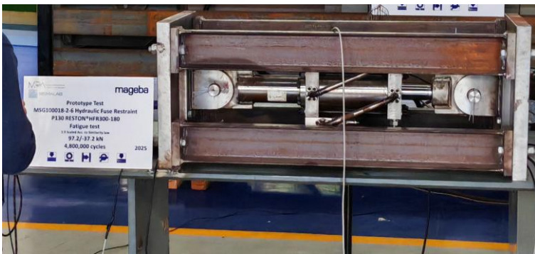
Figure 17: HFR fatigue test - 4,800,000 cycles - scaled
