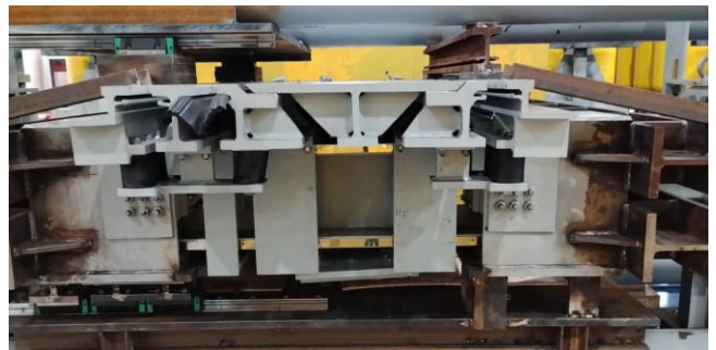
Figure 7: LR3-FE fuse break-away test – more stroke capacity released
