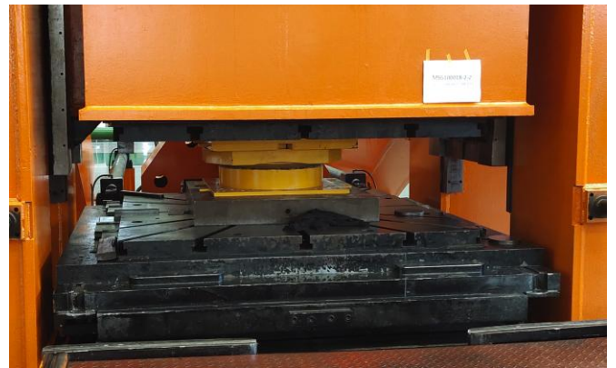
Figure 9: FPB scaled prototype testing
