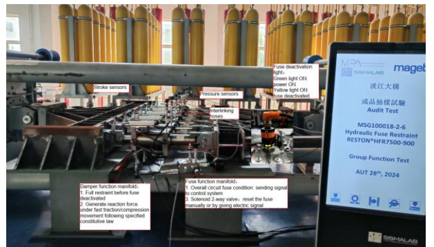
Figure 18: HFR group functioning test - scaled
