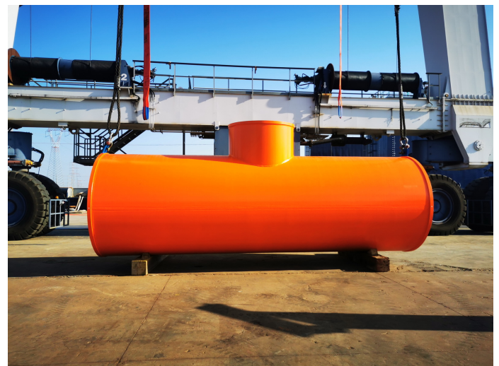
Figures 17 and 18: Tubular monolithic element of the arch, model (left) and final element (right)
