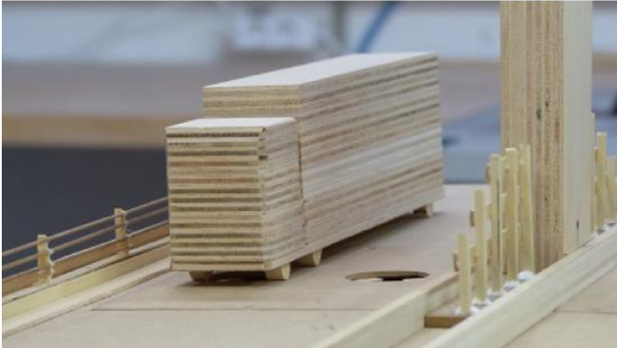
Figure 12: Truck at pylon location in the wind tunnel model
