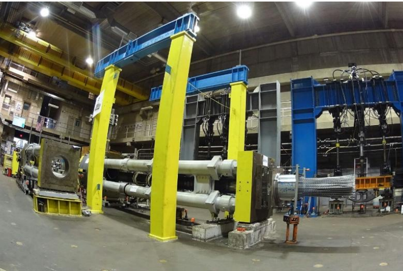
Figure 4: Tensile fatigue and static test set-up over 127-strand SC – CTL, Illinois - USA
