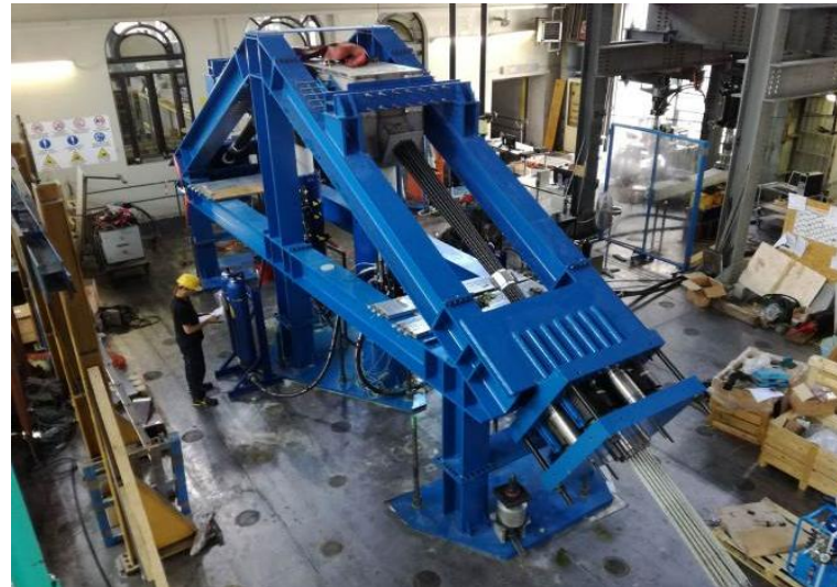
Figure 5: Tensile fatigue and static test set-up over a multi-tube saddle for 37-strand SC – LPM, Politecnico di Milano - Italy
