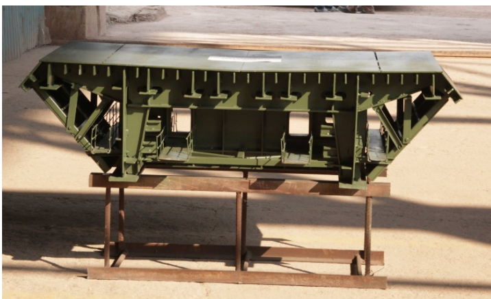
Figure 6: Fabricated steel model for the superstructure
