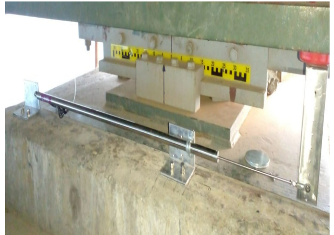
Figure 4: Installed longitudinal and transverse LVDTs
