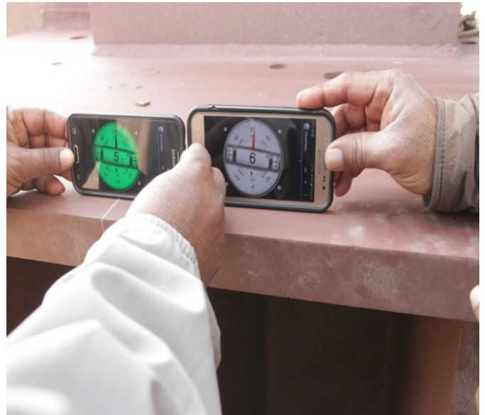
Figure 8: Measurement of inclination
