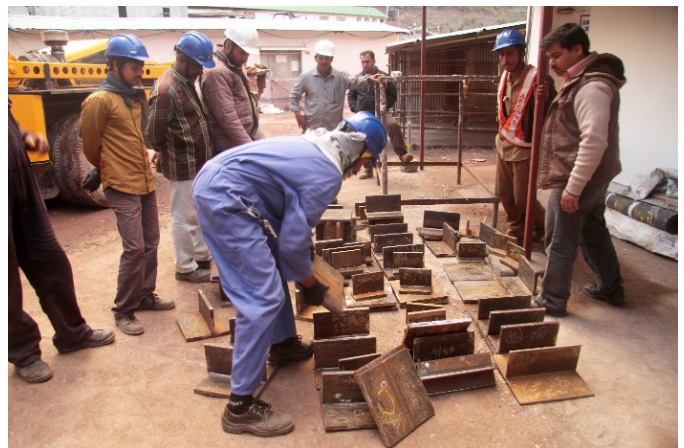
Figure 19: Inspection of the welding pieces
