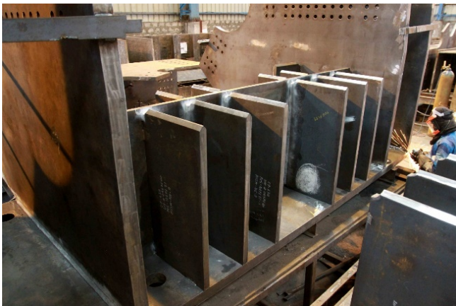
← Figure 39: Heavy stiffeners shall be welded with very small place
