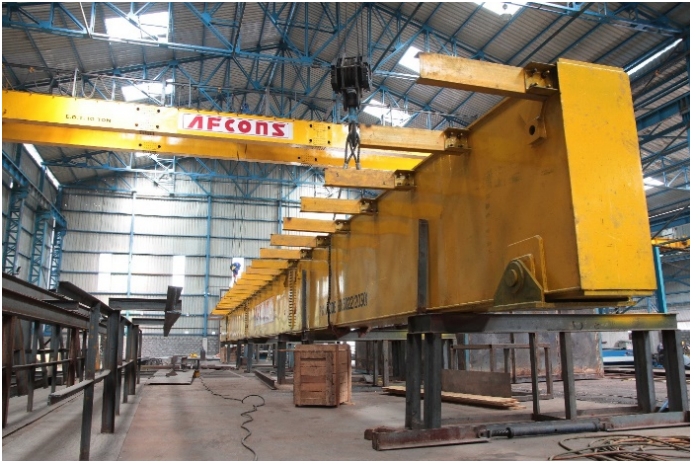
Figure 13: Main girder gantry crane
