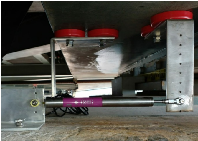
Figure 4: Installed longitudinal and transverse LVDTs
