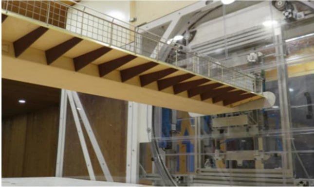
Figure 15: Sectional deck model in wind tunnel (left), wind splitter plate to mitigate VIO (right)
