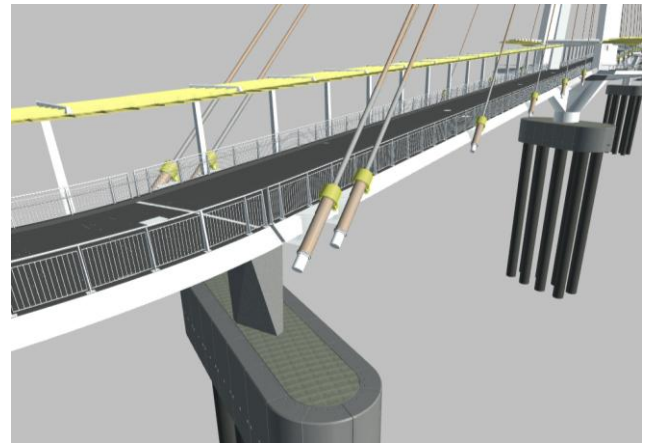
Figure 15: Backstay cable anchorages; FE Analysis of Back Stay Anchors (Concrete Not Shown) (left); Detailed Design Digital Structural Model (right)
