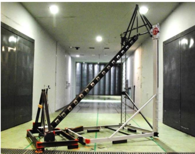
Figure 17: Testing of the integrated stay cable lighting system
