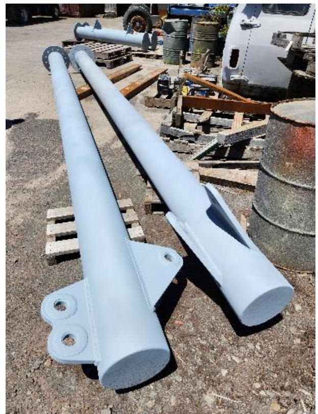
Figure 9: Mast components being fabricated at PACE Engineering, New Plymouth
