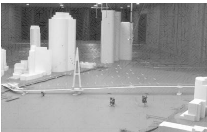
Figure 20: Critical to reliable user comfort is the wind and pedestrian vibration analysis, backed by physical testing under both the completed configuration (left) and during construction (right)
