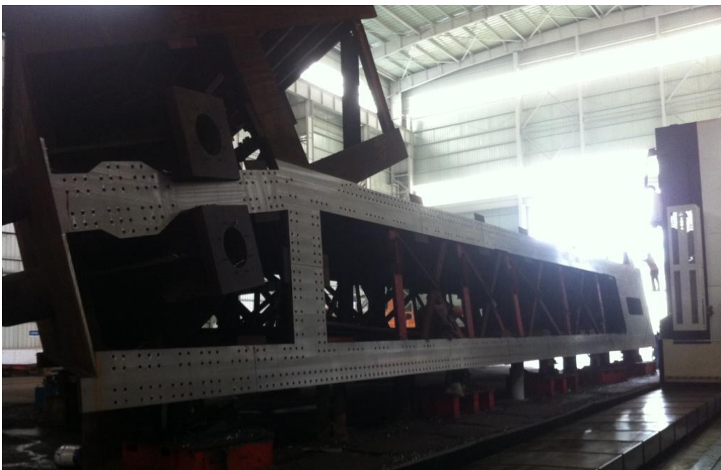
Figure 25: Drilling bolt holes using CNC machine
