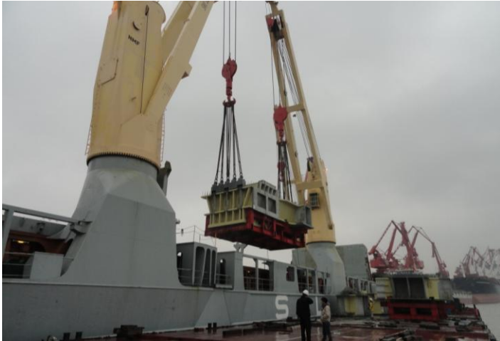
Figure 34: Shifting of segments on a geared vessel
