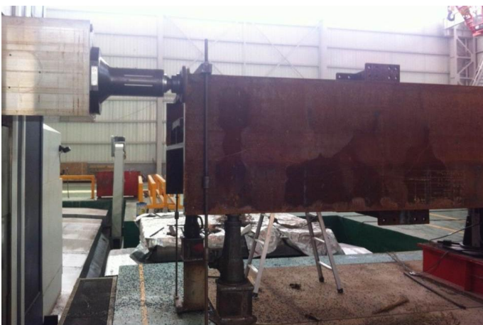
Figure 21: Machining end surface of girder
