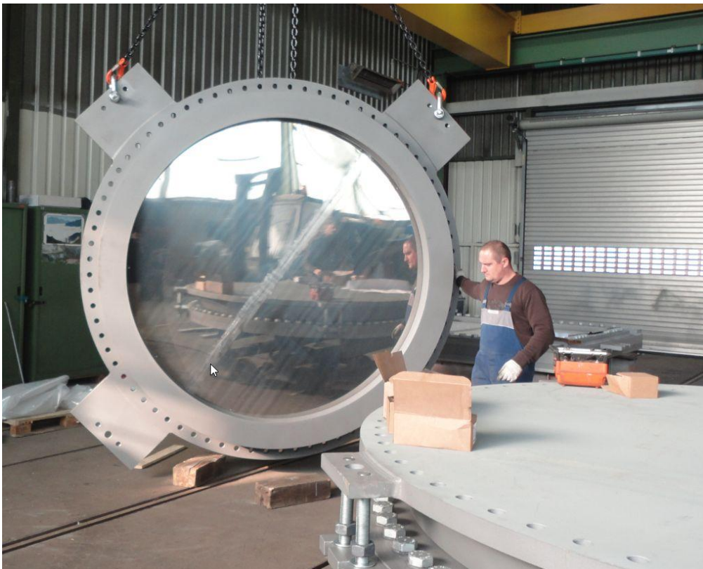
Figure 1: Fabrication of the MAURER MSM® Spherical Bearing
