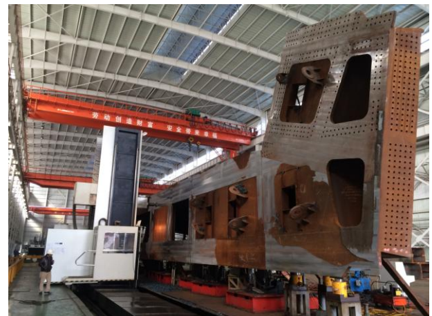
Figure 22: Machining pylon kink 32m long and 7m high
