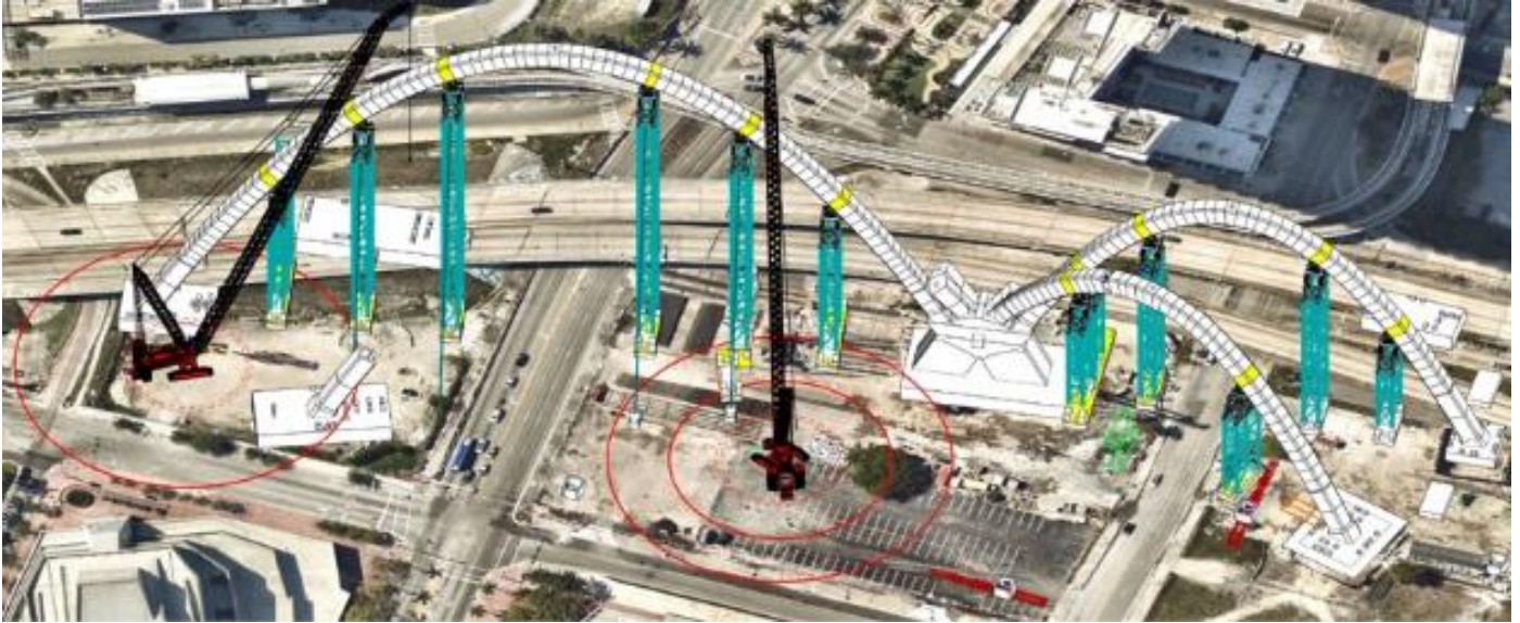
Figure 8: All arch segments are crane erected. This figure shows the 3D modelling used for planning of every crane pick to confirm reach, capacity, and conflict avoidance.
