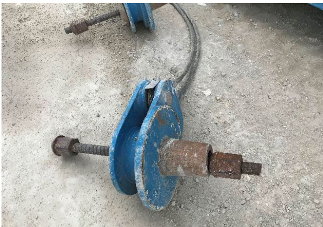
Figure 5: Segment rigging lug. Pre-formed holes on the sides of the precast segments receive the conical insert and the bars are secured by knocker-wrench.
