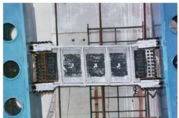
Figure 15: Full scale test of shear link type 1 at University of California at San Diego
