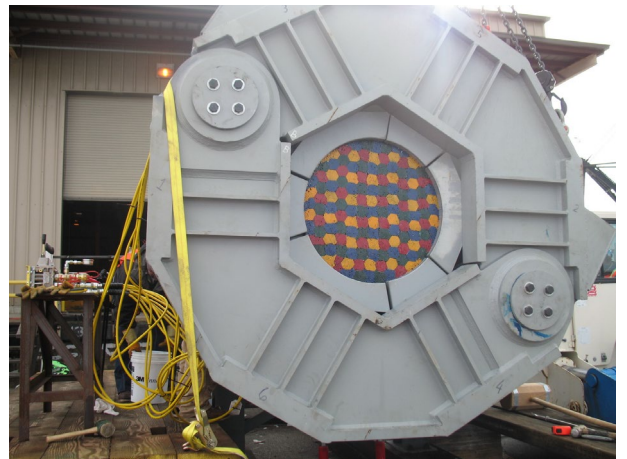
View of cable compactor
