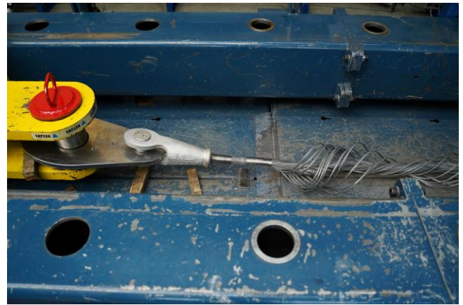
Figure 10: Complete hangers were tested for ultimate load in a static break test
