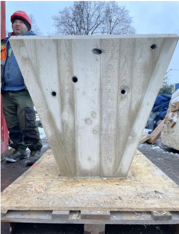
Figure 38: Sampling of concrete and formwork surface
