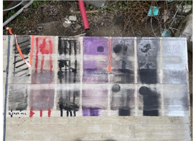
Figure 39: Sampling of anti-graffiti coatings
