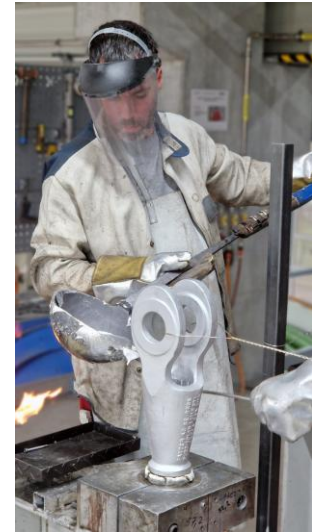
Figures 6 and 7: The sockets have a conical inside, which, for the rope end, opens into a brush to sit in. A special zinc alloy was molten at about 450°C and poured into the inside to form a cone with the wires.
