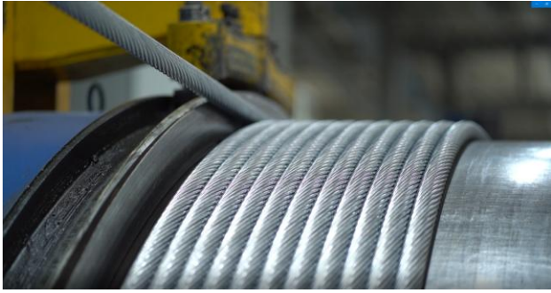
Figure 2: After carefully installing 42 wires into the stranding machine over two days, it took only half a day to manufacture the Menai rope
