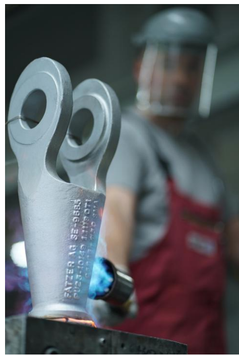
Figure 5: As preparation for the socketing process, the sockets were heated to about 350°C
