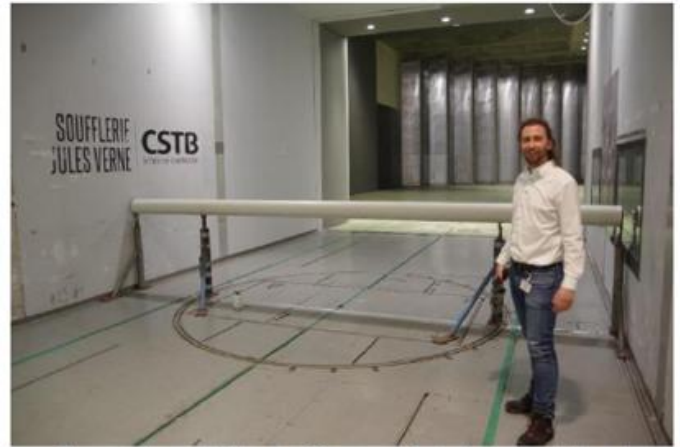
Figure 2: Wind tunnel testing of 200 mm HDPE pipe drag coefficient C_D at CSTB, France
