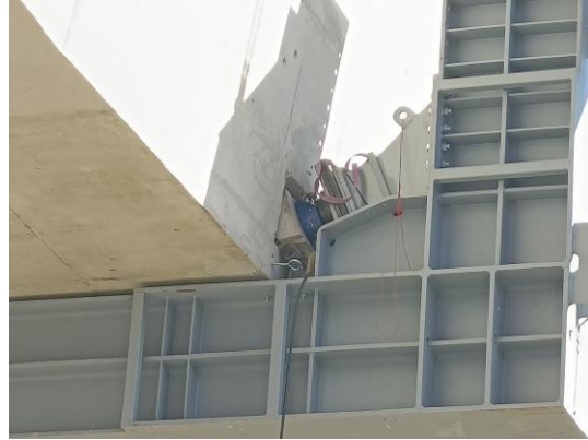
Figures 23 and 24: Load test in strut niches
