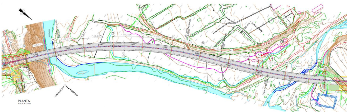
Figure 4: A-23 Sabiñanigo Bridge Span arrangement (plan view) [3]
