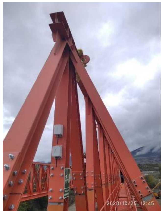
Figure 42: Accelerometer installed at nose tip
