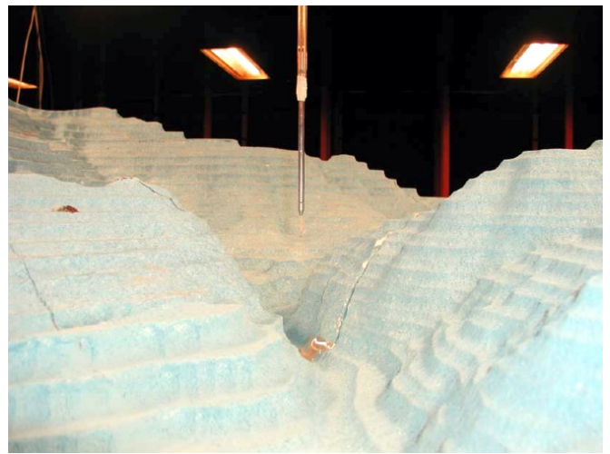
Figure 1: Topography testing: a) computer model b) the scale mode ready for transport c) the model in the wind tunnel and d) hot-wire measurement technology
